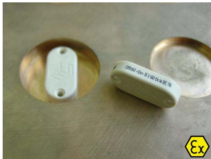
Figure 3. Ferroxtag on screw box ATEX certified re-tuned for metal notch applications.
